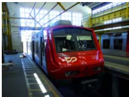
Figure 1: The Siemens 2400 Series EMU introduced in 1992 are targeted for power converter upgrade to extend track life and reliability
