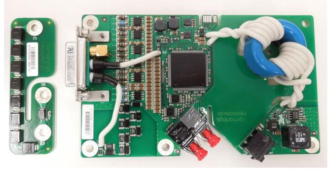
This datasheet describes a 3300V single channel off-module gate drive. The gate drive incorporates protection features for the IGBT module and can be configured by the user for optimised operation in the power stack of the end application. Connection to the IGBT is made with a cable and small module interface card (MIC).
