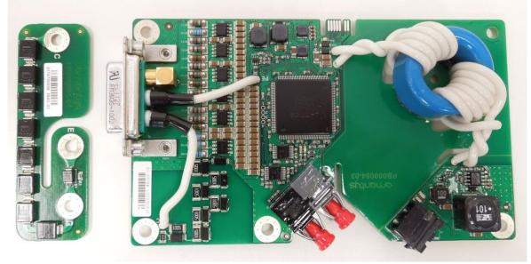
This datasheet describes a 3300V single channel off-module gate drive. The gate drive incorporates protection features for the IGBT module and can be configured by the user for optimised operation in the power stack of the end application. Connection to the IGBT is made with a cable and small module interface card (MIC).
