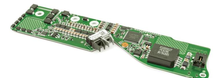
The Amantys Single Channel On-module Gate Drive will drive high power single switch IGBT modules for 2-level and multi-level applications. The gate drive incorporates protection features for the IGBT module and can be configured by the user to optimise the operation of the gate drive in the power stack of the end application. 1200V and 1700V variants are also available.
