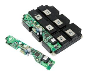
The Amantys AP12A and AP17A are compact, single channel gate drives for high-power IGBT modules. They drive all leading manufacturer's modules and fit within the footprint of the 140x190mm package popular in high power converters, eliminating the need for external mechanical protection.
